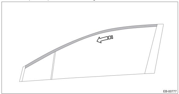
2) Apply the front door sash tape - rear from the top of the vehicle towards the bottom.
