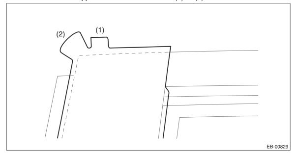
4) Apply the rear door sash tape - rear from the top of the vehicle towards the bottom.
