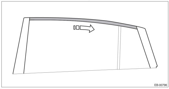
2) Apply the rear door sash tape - front from the top of the vehicle towards the bottom.
