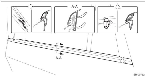
7) Peel the door sash tape from the door sash.
