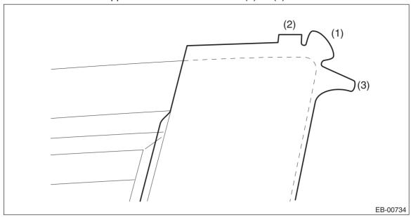
4) Apply the front door sash tape - front from the top of the vehicle towards the bottom.
