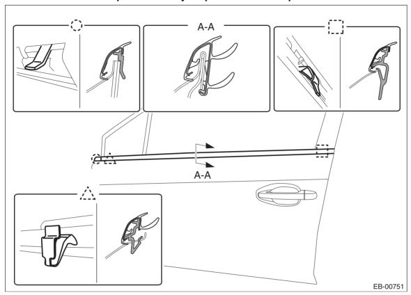
8) Peel the door sash tape from the door sash.
